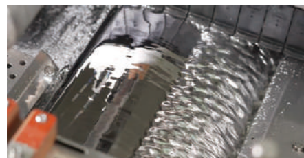
RK Nozzle that inhibits dross adhesion for superior solderability
