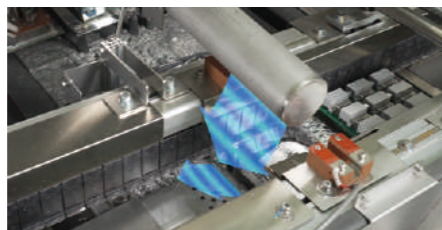
Air Curtain Quenching System for reliable solder solidification
